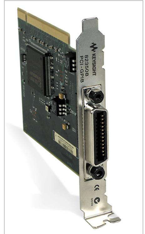
82350B PCI high-performance GPIB interface card
