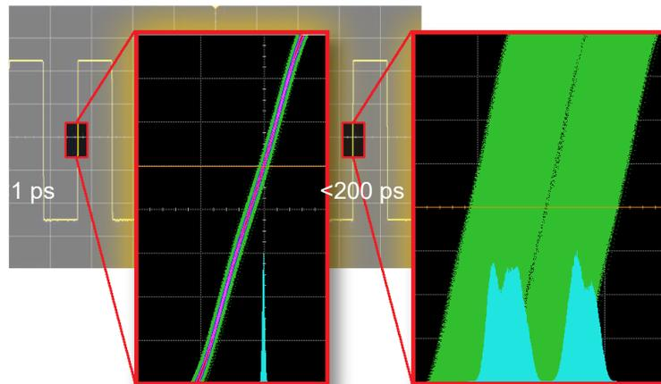
Trueform technology shown on the left significantly improves jitter performance compared to a traditional function generator shown on the right.
