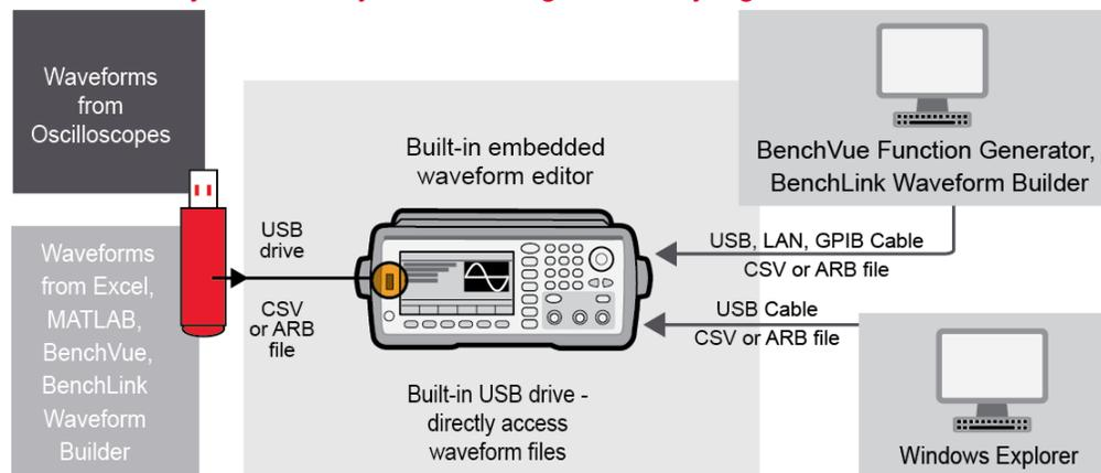
Multiple interfaces provide flexibility for creating and downloading waveforms.
