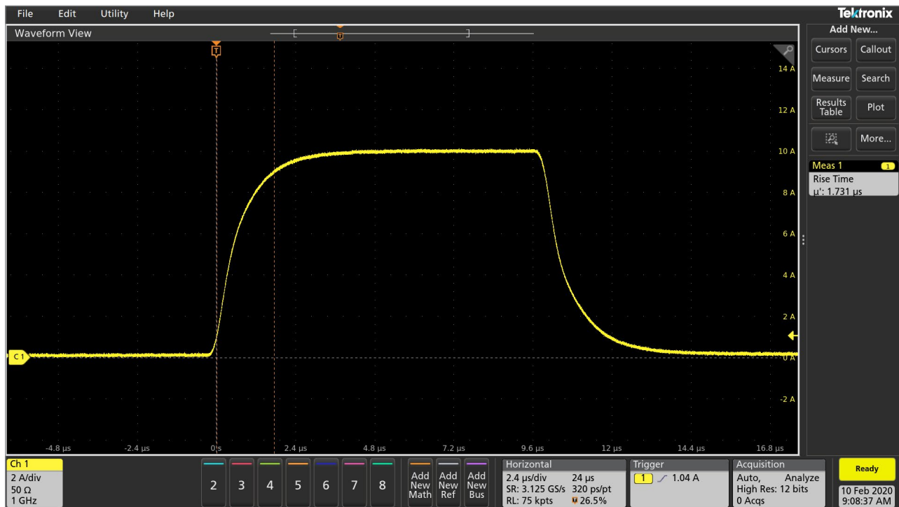
Pulse output performance of the 2610B-PULSE SMU.
