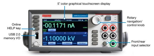
2470 front panel with high-resolution, capacitive touchscreen.
