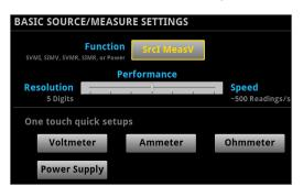
One-touch Quickset modes speed measurement setups nd minimize the time to measurements.
