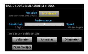
Four "Quickset" modes simplify user setup. With one touch, the instrument can be quickly configured for various operating modes without the need to configure the instrument indirectly for this operation.
