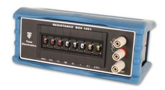
The **1051** is a wide range low ohm resistance box designed for general laboratory work including platinum resistance thermometry.
